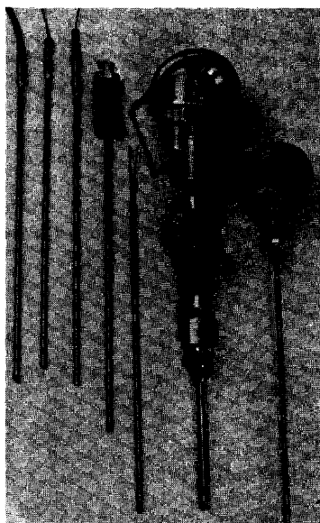
Figure 3.17 Thermocouple types. (Courtesy The Foxboro Co. ) (a) Wire type. (b) PYOD type. (c) Minox type.
