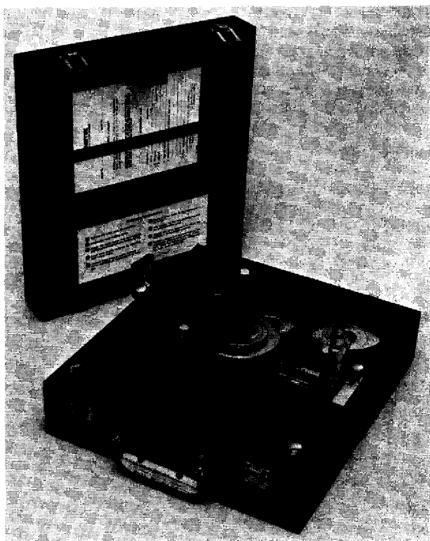
Figure 3.9 Pneumatic deadweight tester. (Courtesy Ametek.)
